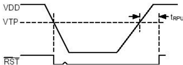
Figure 2. Low Voltage Reset
