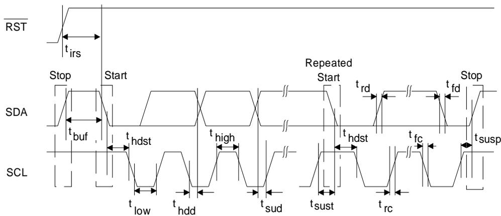
**Figure 3. I<sup>2</sup>C Control Port Timing**
