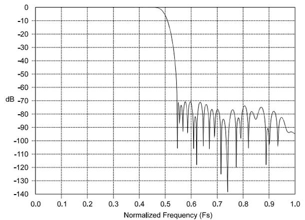
**Figure 20. DAC Filter Response**
