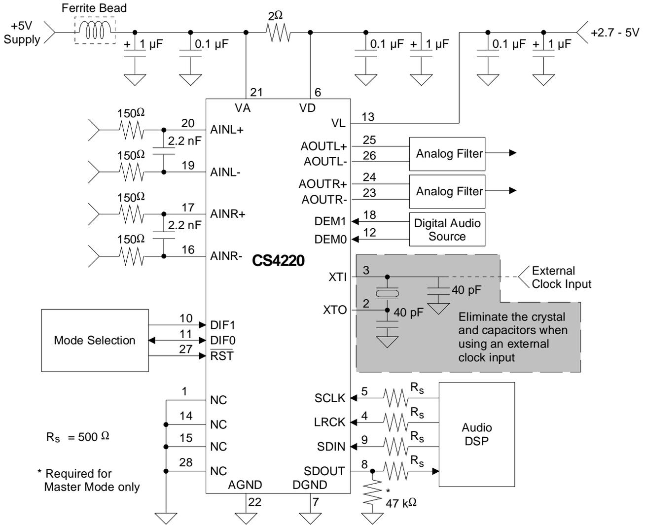
**Figure 4. CS4220 Recommended Connection Diagram**
