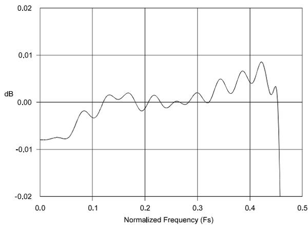
**Figure 21. DAC Passband Ripple**
