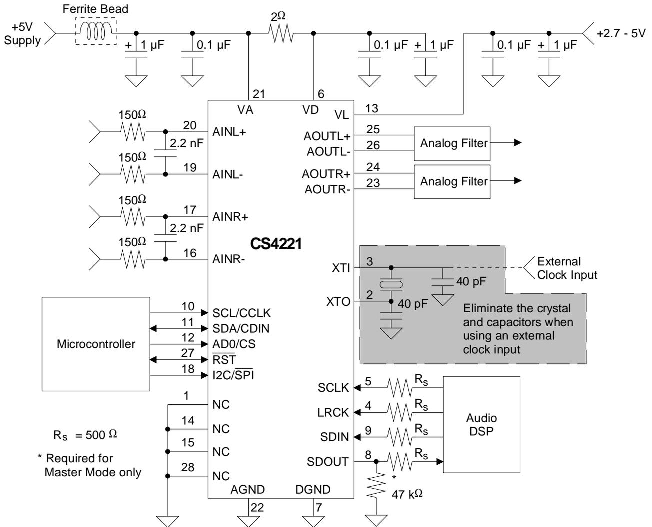
**Figure 5. CS4221 Recommended Connection Diagram**
