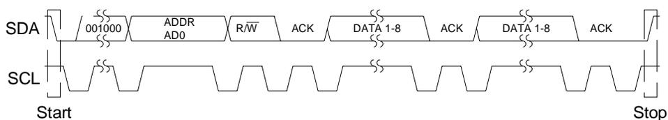
**Figure 7. Control Port Timing, I<sup>2</sup>C mode**
