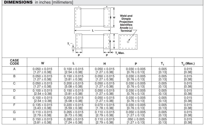
Note: When solder coated terminations are required, add 0.015" [0.381] to termination dimension tolerances.
