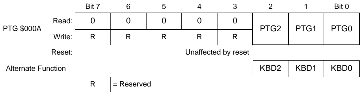
Figure 19-19. Port G Data Register (PTG)
