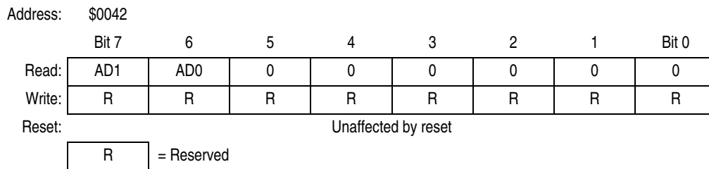
Figure 3-7. ADC Data Register Low (ADRL) Left Justified Mode
