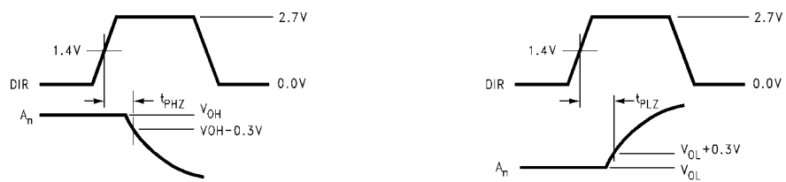
FIGURE 7. t_{pHZ} and t_{pLZ} Test Load and Waveforms, DIR to A_1-A_8
