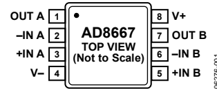
Figure 1. 8-Lead MSOP, 8-Lead SOIC
