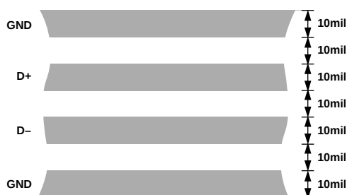
Figure 14. Arrangement of Signal Tracks
