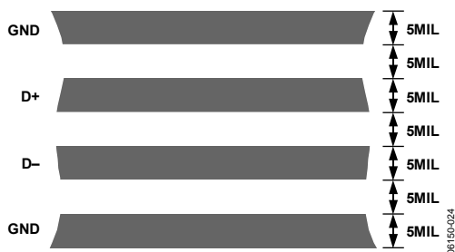
Figure 24. Typical Arrangement of Signal Tracks
