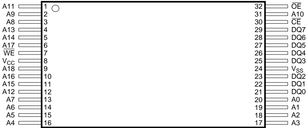
29F040 Standard Pinout
