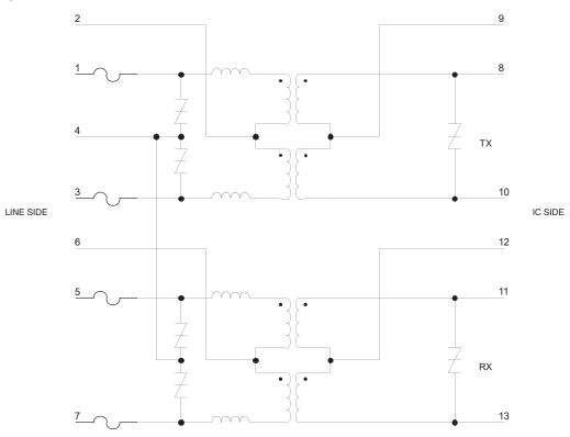
INCLUDES: ISOLATION TRANSFORMERS, COMMON MODE CHOKE, PROTECTION COMPONENTS (LINE AND CHIP SIDE)
