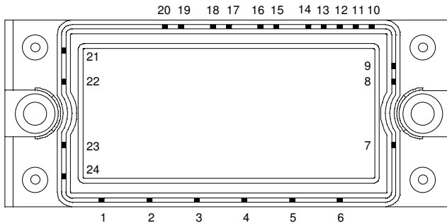
APTGF20X60RTP2: Without Brake (Pin 7 & 14 not connected)
