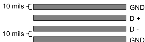
Figure 13 Recommended Remote Diode Circuit Board Interconnect
