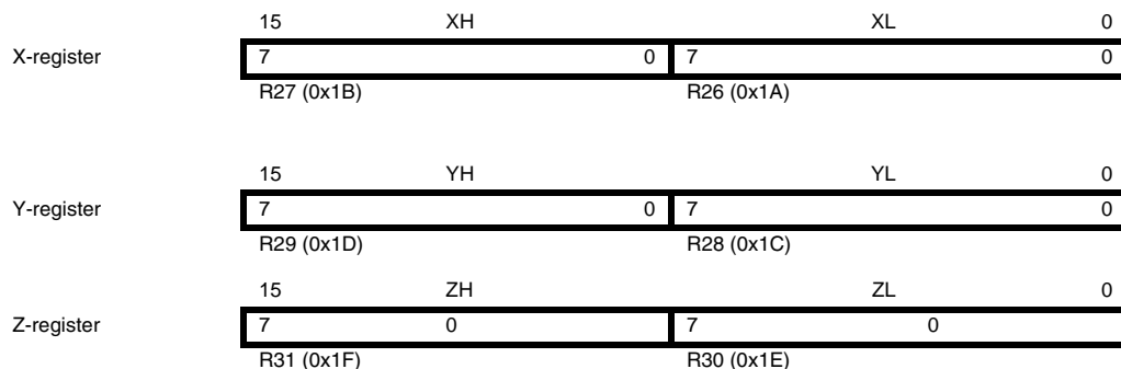
Figure 5. The X-, Y-, and Z-registers
