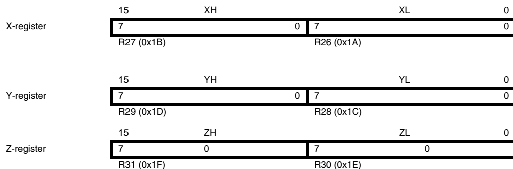
Figure 5. The X-, Y-, and Z-registers
