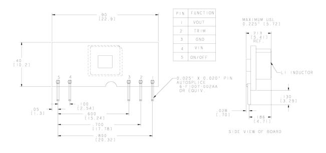
BOTTOM VIEW OF BOARD ALL DIMENSIONS ARE IN INCHES [MM].
