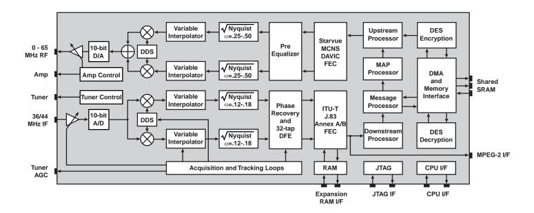
The Broadcom® BCM3300 combines a 256-QAM receiver, a 4/16-QAM burst transmitter and a complete DOCSIS compliant MAC integrated into a single chip. The BCM3300 is the world's first and only single chip, DOCSIS version 1.0 and 1.1 compliant solution with extensions for fragmentation and Quality of Service (QoS).
