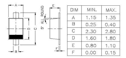
All dimensions are in mm CATHODE IS MARKED BY BAND
