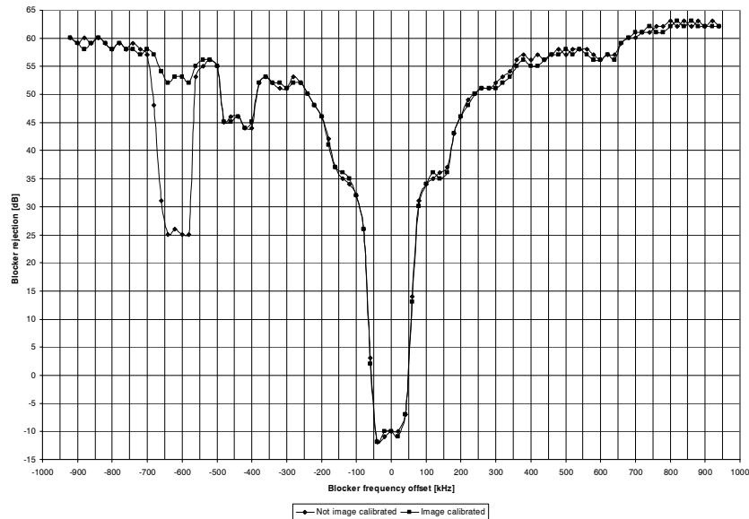
Figure 19. Typical blocker rejection. Carrier frequency set to 868.3072 MHz (102.4 kHz channel filter bandwidth, 38.4 kBaud)
