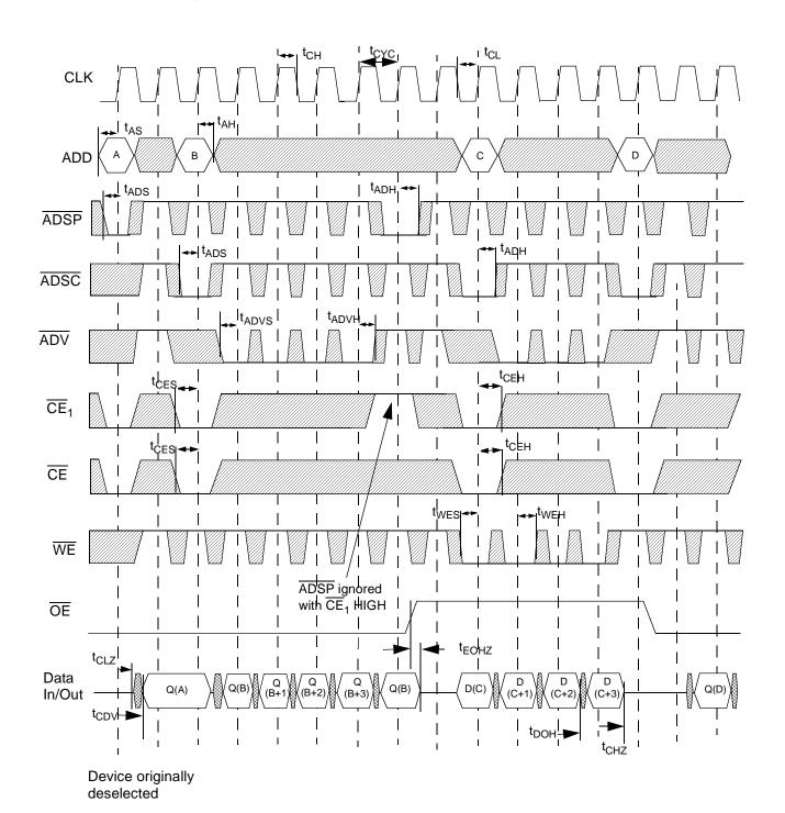
$\overline{\text{WE}}$  is the combination of  $\overline{\text{BWE}}$ ,  $\overline{\text{BWS}}_{[1:0]}$ , and  $\overline{\text{GW}}$  to define a write cycle (see Write Cycle Descriptions table).  $\overline{\text{CE}}$  is the combination of  $\overline{\text{CE}}_2$  and  $\overline{\text{CE}}_3$ . All chip selects need to be active in order to select the device. RAx stands for Read Address X, WAx stands for Write Address X, Dx stands for Data-in X, Qx stands for Data-out X.
