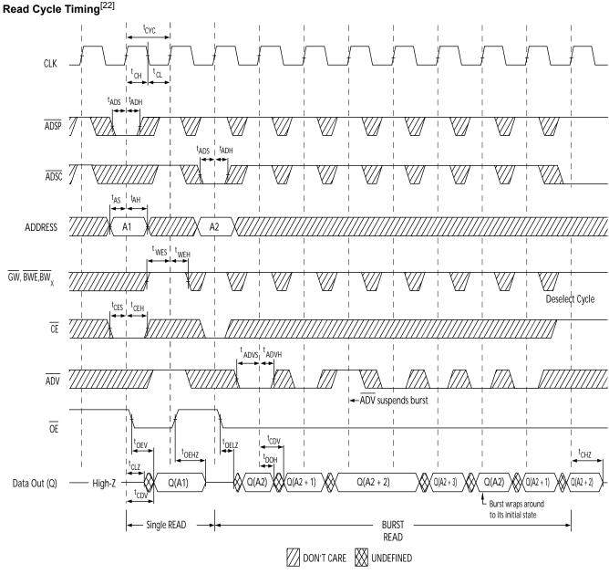
Note: 22. On this diagram, when  $\overline{CE}$  is LOW:  $\overline{CE}_1$  is LOW,  $\overline{CE}_2$  is HIGH and  $\overline{CE}_3$  is LOW. When  $\overline{CE}$  is HIGH:  $\overline{CE}_1$  is HIGH or  $\overline{CE}_2$  is LOW or  $\overline{CE}_3$  is HIGH.
