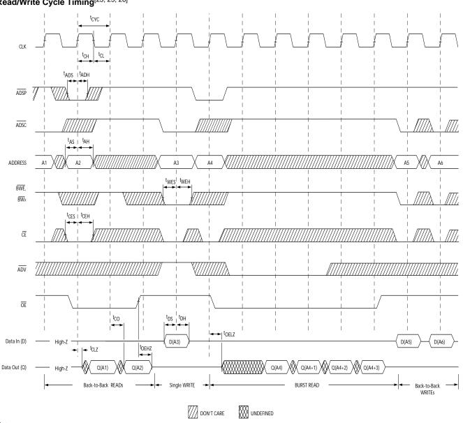
25. <u>The</u> data bus (Q) remains in high-Z following a Write cycle, unless a new Read access is initiated by ADSP or ADSC. 26. GW is HIGH.
