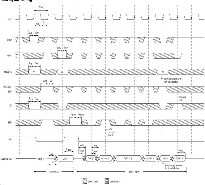
Note: 23. On this diagram, when  $\overline{\text{CE}}$  is LOW:  $\overline{\text{CE}}_1$  is LOW,  $\overline{\text{CE}}_2$  is HIGH and  $\overline{\text{CE}}_3$  is LOW. When  $\overline{\text{CE}}$  is HIGH:  $\overline{\text{CE}}_1$  is HIGH or  $\overline{\text{CE}}_2$  is LOW or  $\overline{\text{CE}}_3$  is HIGH.
