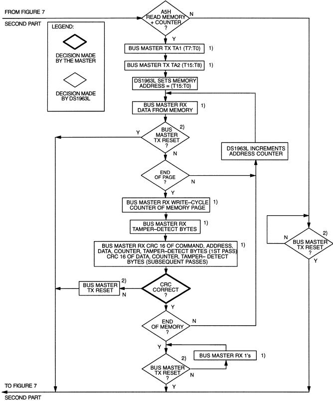
1) To be transmitted or received at Overdrive Speed if OD = 1
