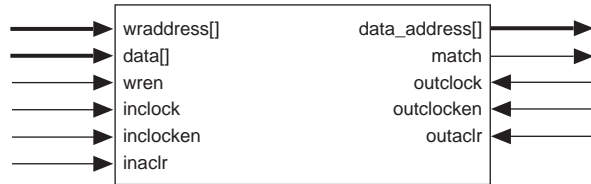
Figure 23. APEX 20KE CAM Block Diagram
