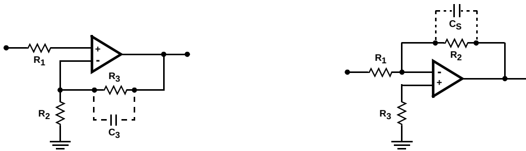
FIGURE 3. SUGGESTED OFFSET VOLTAGE ADJUSTMENT
