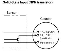
Solid-State Input (NPN output sensor powered by built-in DC power source)
