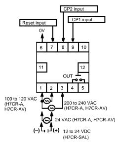
Single Preset Transistor (NPN) Output
