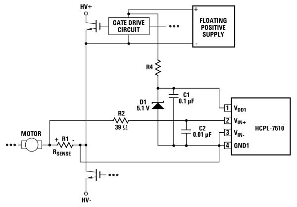
Figure 16. Recommended supply and sense resistor connections.
