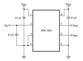
Figure 12. Propagation delay test circuit.
