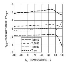
Figure 13. Propagation delay vs. temperature.
