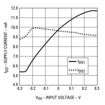
Figure 3. Supply current vs. input voltage.
