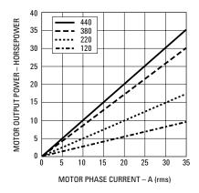
Figure 18. Motor output horsepower vs. motor phase current and supply voltage.
