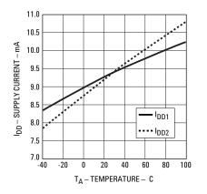
Figure 2. Supply current vs. temperature.
