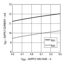
Figure 1. Supply current vs. supply voltage.
