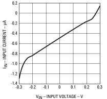
Figure 4. Input current vs. input voltage.
