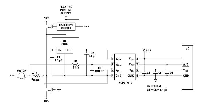
Figure 17. Recommended HCPL-7510 application circuit.
