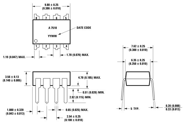
DIMENSIONS IN MILLIMETERS AND (INCHES). NOTE: FLOATING LEAD PROTUSION IS 0.5 mm (20 mils) MAX.
