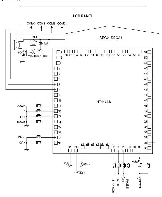
Notes: The IC substrate should be connected to VSS in the PCB layout artwork.
