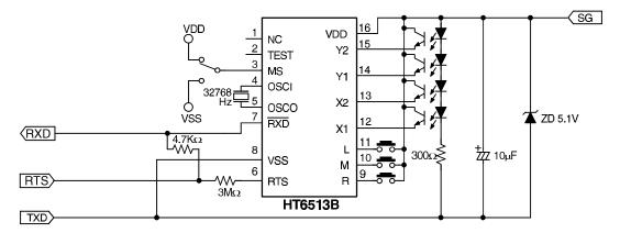
The  $\overline{\mbox{RXD}}$  pin is NMOS open drain output.
