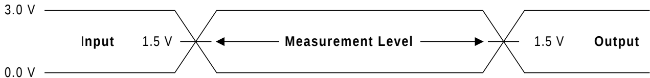
Figure 14. Input Waveforms and Measurement Levels
