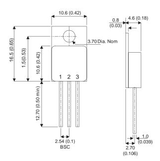
N-Channel MOSFET in a Hermetically sealed TO257AB Metal Package.
