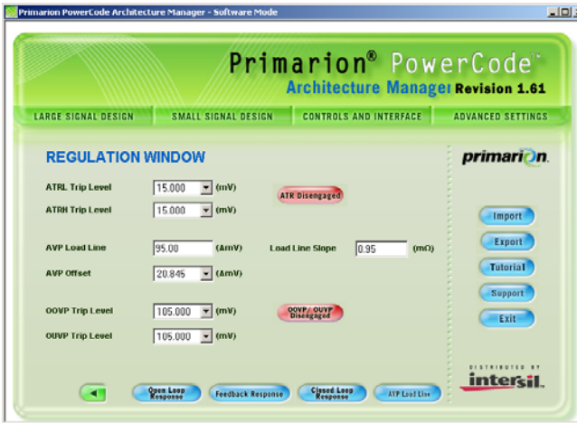
FIGURE 23. PRIMARION POWERCODE LOADLINE AND ATR SETTINGS
