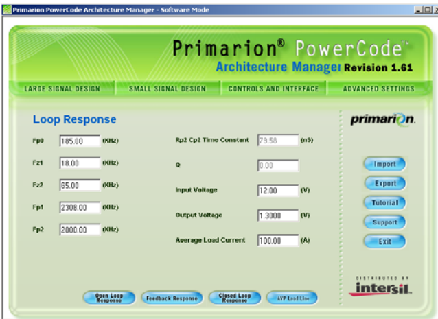
FIGURE 24. PRIMARION POWERCODE LOOP RESPONSE SETTINGS
