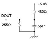
\* Including Scope and Jig Capacitance
