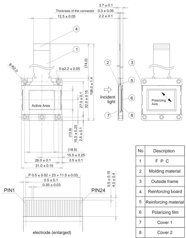
The rotation angle of the active area relative to H and V is  $\pm 1^{\circ}$ .
