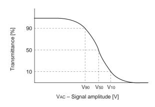
Input signal voltage (Waveform applied to the measured pixels)
