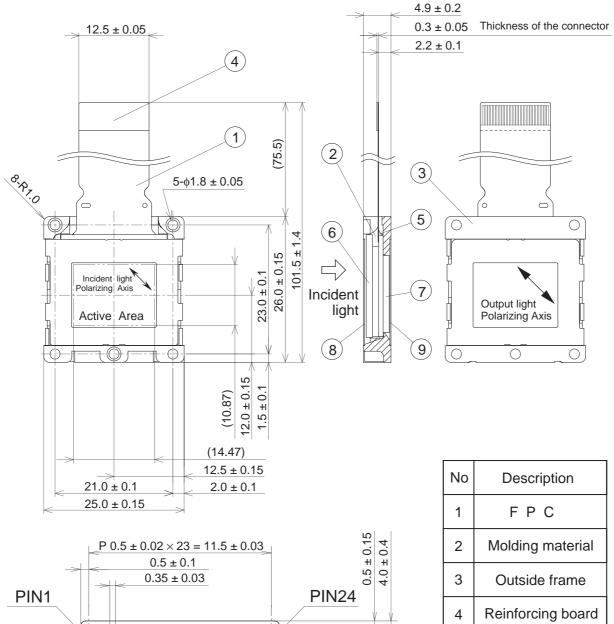
The rotation angle of the active area relative to H and V is  $\pm 1^{\circ}$ .
