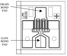
DIE SIZE: 15.4X14.2 mils (390x360 μm) DIE THICKNESS: 3.9 mils (100 μm) BONDING PADS: 3.0X3.0 mils (75x75 μm)
