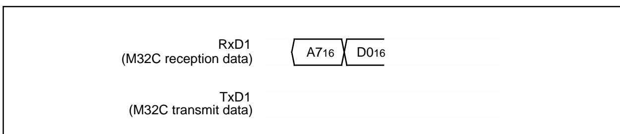
Figure 1.35.27. Timing for erasing all unlocked blocks
