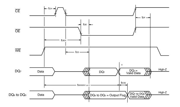
(5) AC Waveforms for Data Polling during Embedded Algorithm Operations
