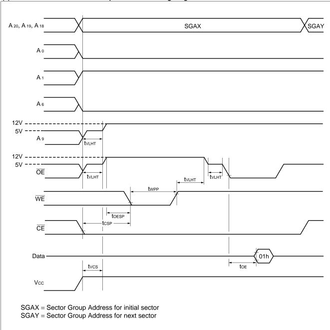
(9) AC Waveforms for Sector Group Protection Timing Diagram
