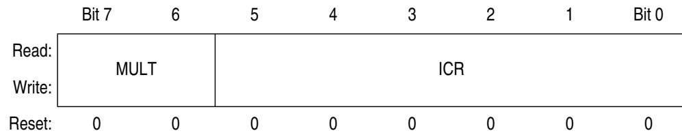
Figure 13-6 IIC Frequency Divider Register (IICF)
