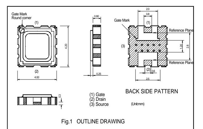
MGF0918A S PARAMETERS (Ta=25°C, VD=10V, ID=150mA, Reference Plane see Fig.1)
