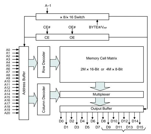
In 8-bit output mode, these pins are placed in a high-Z state and pin D15 functions as the A-1 address pin.
