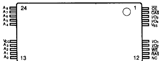
20/24-pin TSOP TYPE ( I ) Reverse Bend (6X16mm) P24TV-5B4-R
