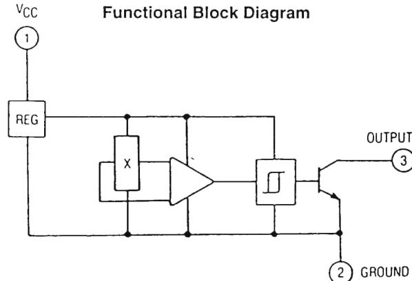
These devices turn on (logic level "0") in the presence of a magnetic south pole and turn off (logic level "1") when subjected to a magnetic north pole. Both magnetic poles are necessary for operation so they are referred to as Bipolar or Latching. This feature makes these sensors ideal for application in brushless DC motors and for use with multiple pole magnets.
