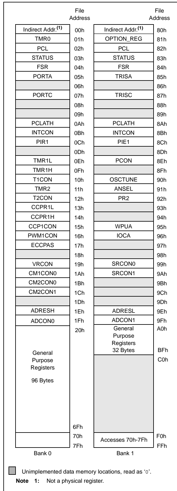
FIGURE 2-2: DATA MEMORY MAP OF THE PIC16F616/16HV616
