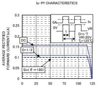
CASE TEMPARATURE:Tc(°C) Derating Curve (Io-Tc)
