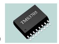
The LF base station IC TMS3705ADR allows efficient development and production of RFID readers for vehicle immobilizers. This base station
