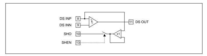
The output of the data slicer (DS-OUT) is a CMOS compatible bitstream. However, it is recommeded that an external NPN amplifier stage be used to drive the CMOS baseband processor, in order to minimize the amount of ground and supply currents in the S1T8531 which might desensitize the chip.
