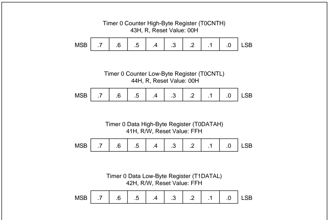
Figure 13-3. Timer 0 Counter and Data Registers (T0CNTH/L, T0DATAH/L)
