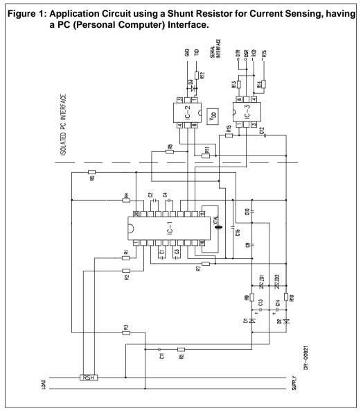
Note: The Serial Interface having a RS232 protocol, has been designed to operate directly with a PC (Personal Computer).
