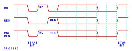
Read, Reset and Read/Reset of integrator for active energy
