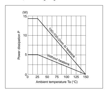
When selecting a heatsink for SLA5017, be sure to check the product temperature when in use in an actual application.
